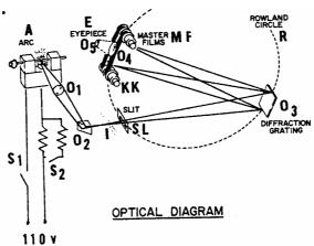
The above diagram illustrates just how a spectrogram of a sample is placed in juxta0position with two continuous spectra by which the standard spectrograms are illuminated.
