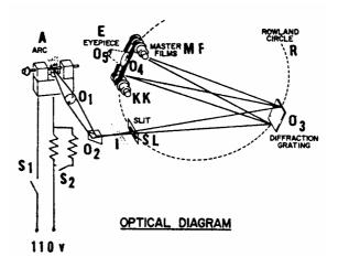
A is an arc holder, with a disposable refractory hearth on which the sample is placed. S1 is a switch for turning the arc on and off. E is an eyepiece by which the spectrum is magnified and viewed. MF are mylar films on which the master spectra are recorded, placed on both sides of the observed spectrum for direct comparison. KK are knobs for turning the spools on which the master spectrum films are wound.
