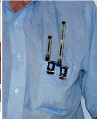
Two units using charcoal and calorimetric tubes - saves cost of charcoal tube analysis if color tube is negative.
