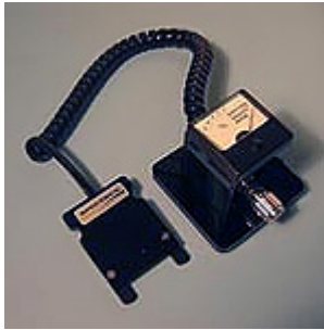
Opacity Meter - provides an instantaneous measurement of the sample's opacity to correlate with computer calculations
