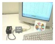
The DL-3 is a custom modified data logger configured for Eco Sensors instruments and applications. It plugs into the accessory jack of the <u>C-30ZX</u> or the <u>C-21</u> to log data without further adjustments. It can download logged data into a PC or laptop by its RS-2 32 serial cable, or it can send data continuously to the PC for continuous display and analysis by the PC.
