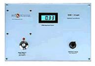
Using proprietary technology, our instrument strips the ozone from the water stream and reads it as the concentration of ozone released into a measuring chamber. This has advantages over conventional methods for measuring dissolved ozone.
