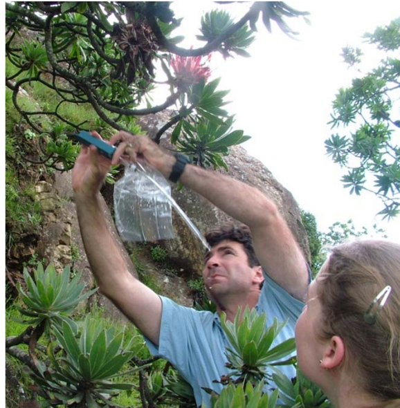
Robert Raguso uses a Spectrex, Inc. PAS-500 portable vacuum pump to collect floral volatiles from a South African Protea tree.
