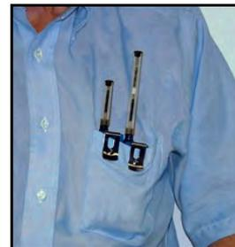
Two units using charcoal and colorimeter tubes - saves cost of charcoal tube analysis if color or tube is negative.
