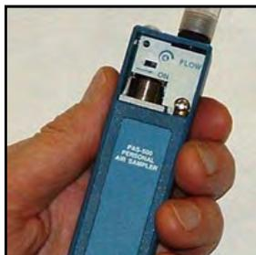
The 9-volt battery easily slips in and out.
